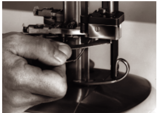
Figure 9. Adjusting Bevel Bloc Shoes
